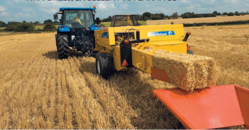
Producing consistent firm bales is a major benefit of the new BC5000 balers. The long bale chamber, allowing for a long plunger stroke, combined with the high plunger speed, ensures a 1<sup>st</sup> class quality bale formation. Adjustable top and bottom bale chamber rails and adjustable bale case doors allow for a perfect setting of the required density.
