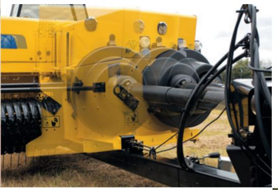
Fast and sure changing from road position to working position is performed with the "hydro swing" drawbar. It uses the tractor hydraulics and makes switching fast and easy.
